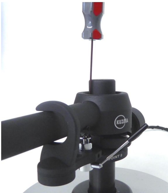
Fig. 12. Adjusting VTA screw
